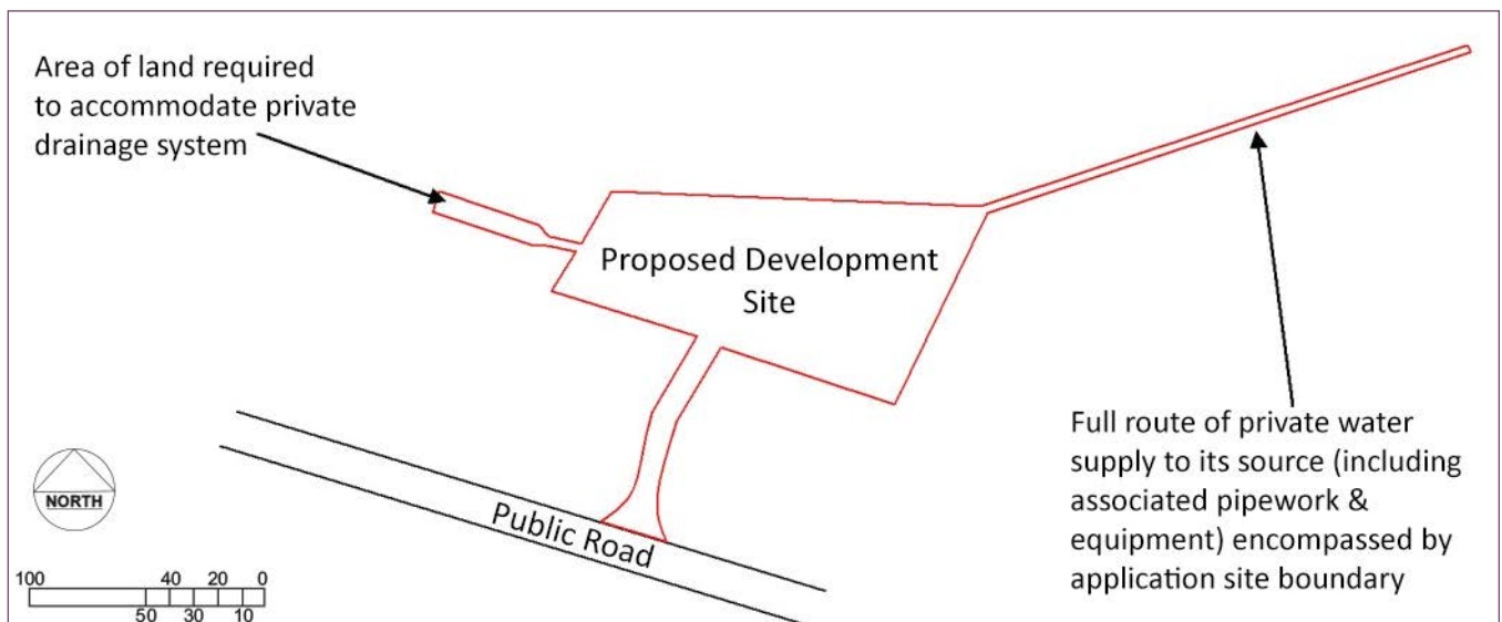
Fig 7. New private water supply and drainage arrangements
