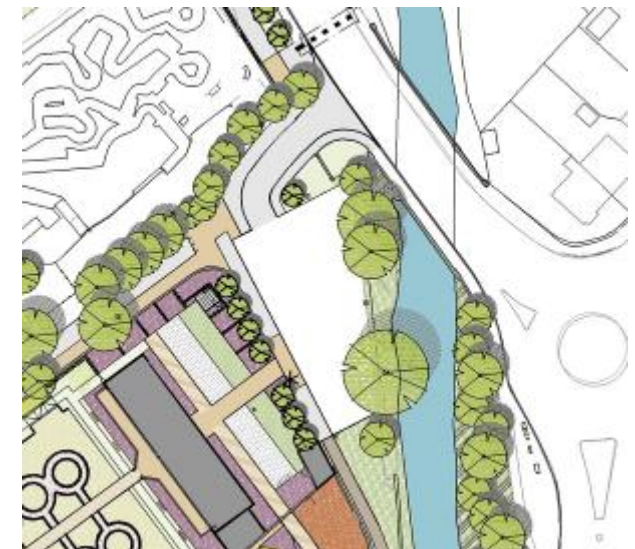
East Entrance with improvements to the visibility splay and enhanced sense of arrival from the road.
