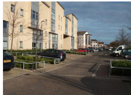
Access Control with street furniture
