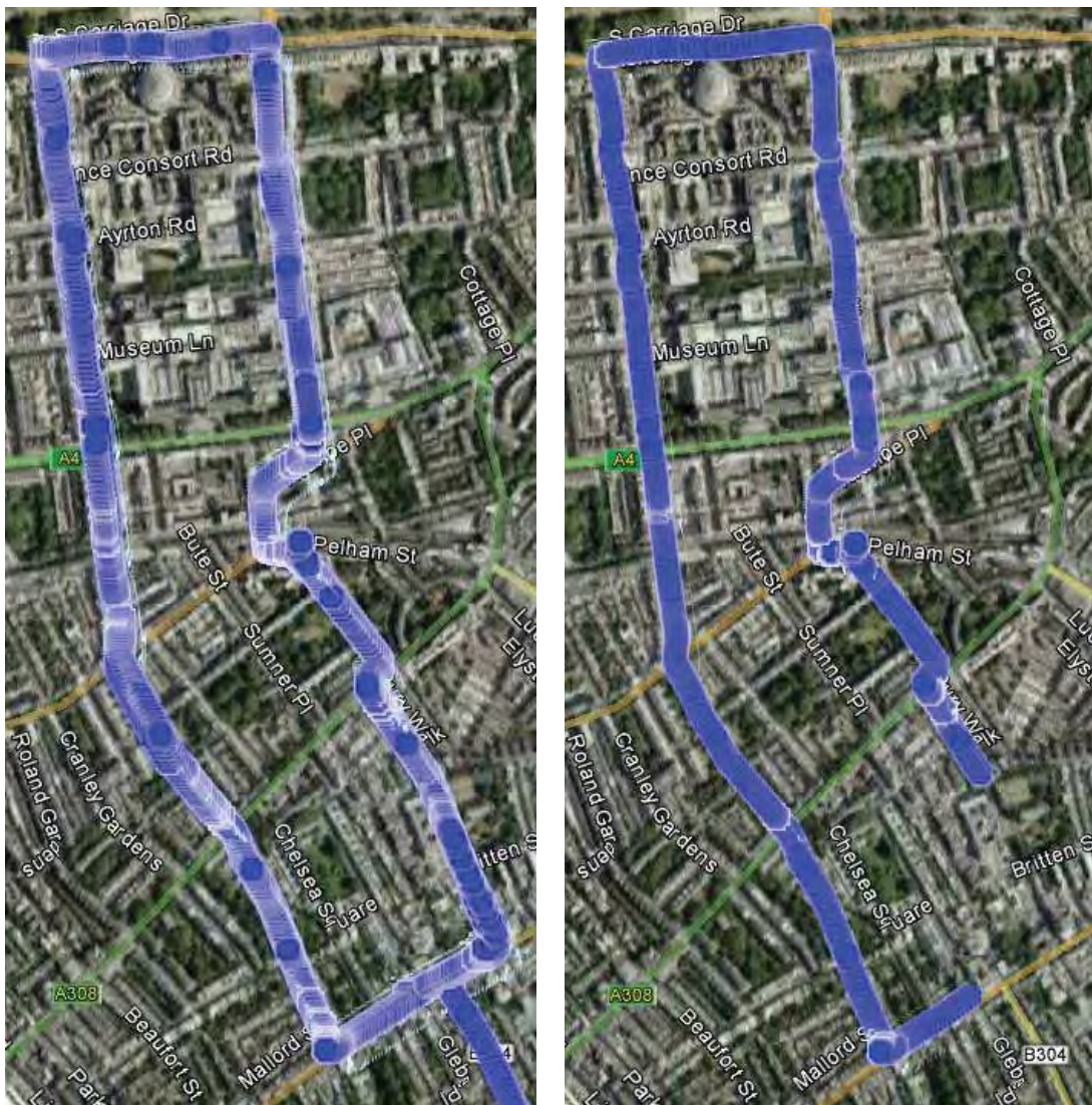
Figure 7: Vehicle trajectory data before and after processing (route F) (map data © Google)
