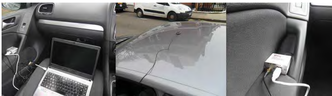
Photograph 1 (L-R): logging setup; antenna position; GPS module
