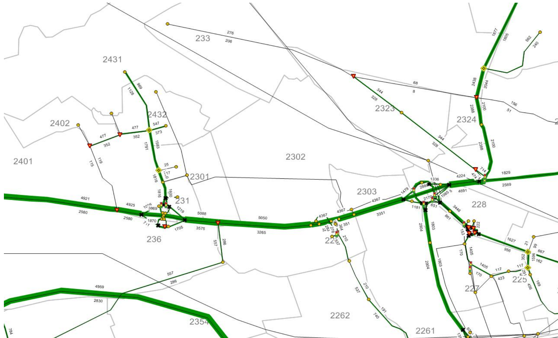
Figure 7.4: Base 2015 AM 2hr link flows (07:00-09:00)
