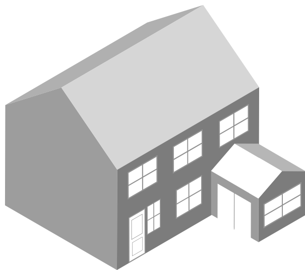
Extension subservient to original home in scale and size and compatible with original house in materials and form
