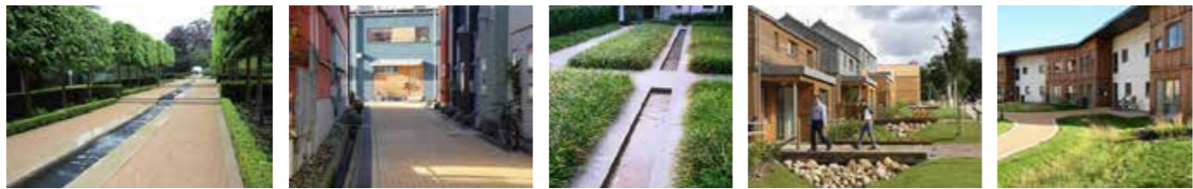
Fig. 3.18: Examples of blue-green infrastructure swales
