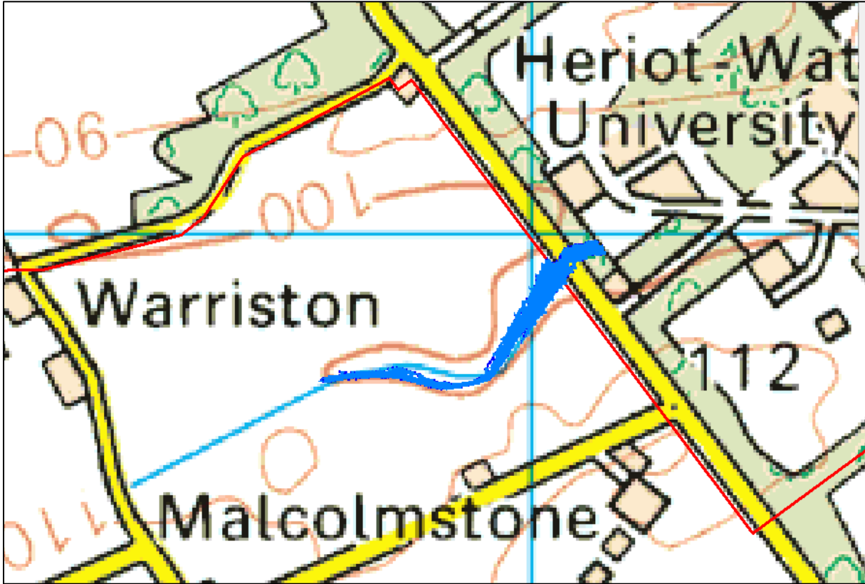
Figure 7. 200 year and 200 year + 30% floodplains for the Unnamed Watercourse (both are approximately the same)
