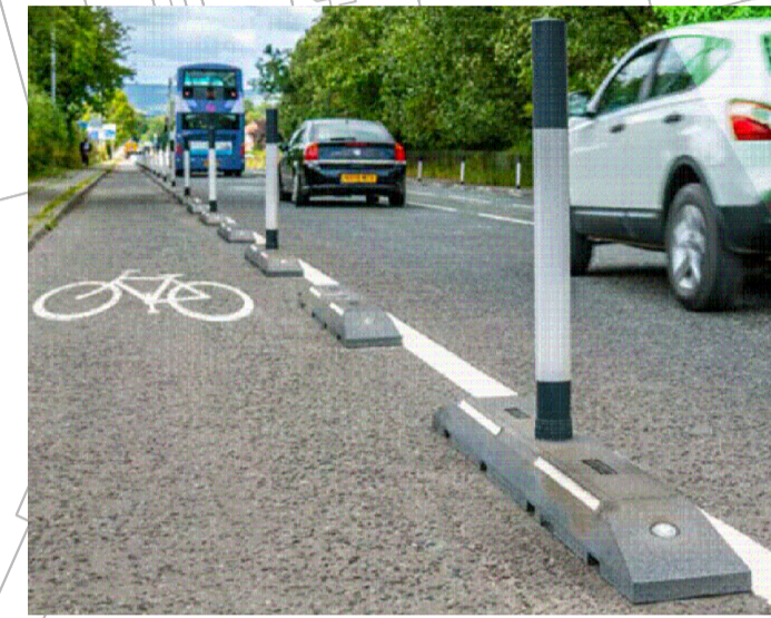
Fig 1. ROSEHILL NARROW CYCLE LANE DEFENDER UNITS - TO PROVIDE TRAFFIC SEGREGATION. PRODUCT 2.0m IN LENGTH & ARE BOLTED INTO CARRIAGEWAY WITH 5m GAP. NOTE DEFENDER TO BE POSITIONED OFFSET 1.5m FROM KERB WITH CONTINUOUS WHITE LINING AT 1.8m OFFSET FROM KERB.
