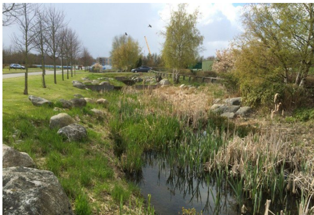
Figure 13. Wet swale populated with invasive bull rush, Heriot Watt Campus | SNH
