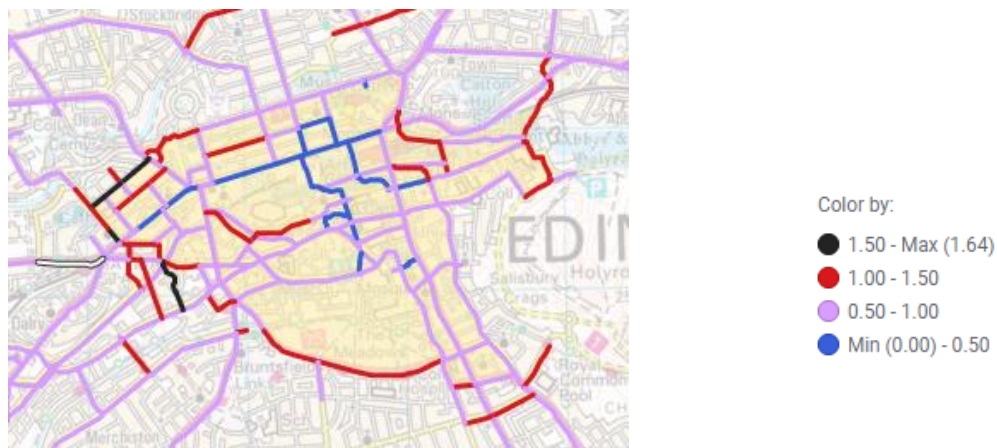
Figure 23: Ratio of Emission Changes (2023) due to introduction of Large LEZ. Black is largest % increase in emissions (> 50%)
