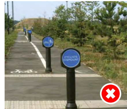
Image: Designing Streets . Over utilisation of signage on cyclist/ pedestrian paths should be avoided.
