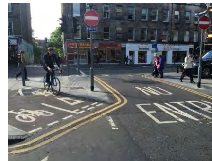
Contraflow cycle lane, Rankeillor Street, Edinburgh (City of Edinburgh Council)
