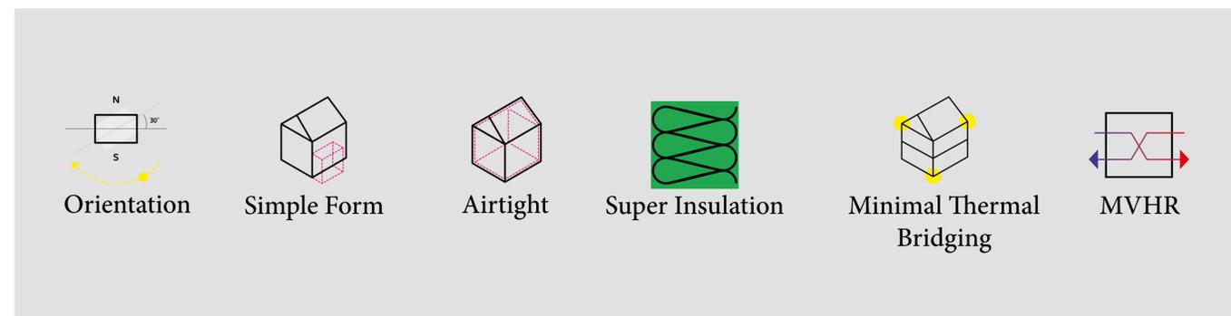
Diagram illustrating key Passivhaus principles
