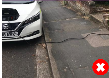
Figure F8.23 - Cable running across the footway, creating a trip hazard
