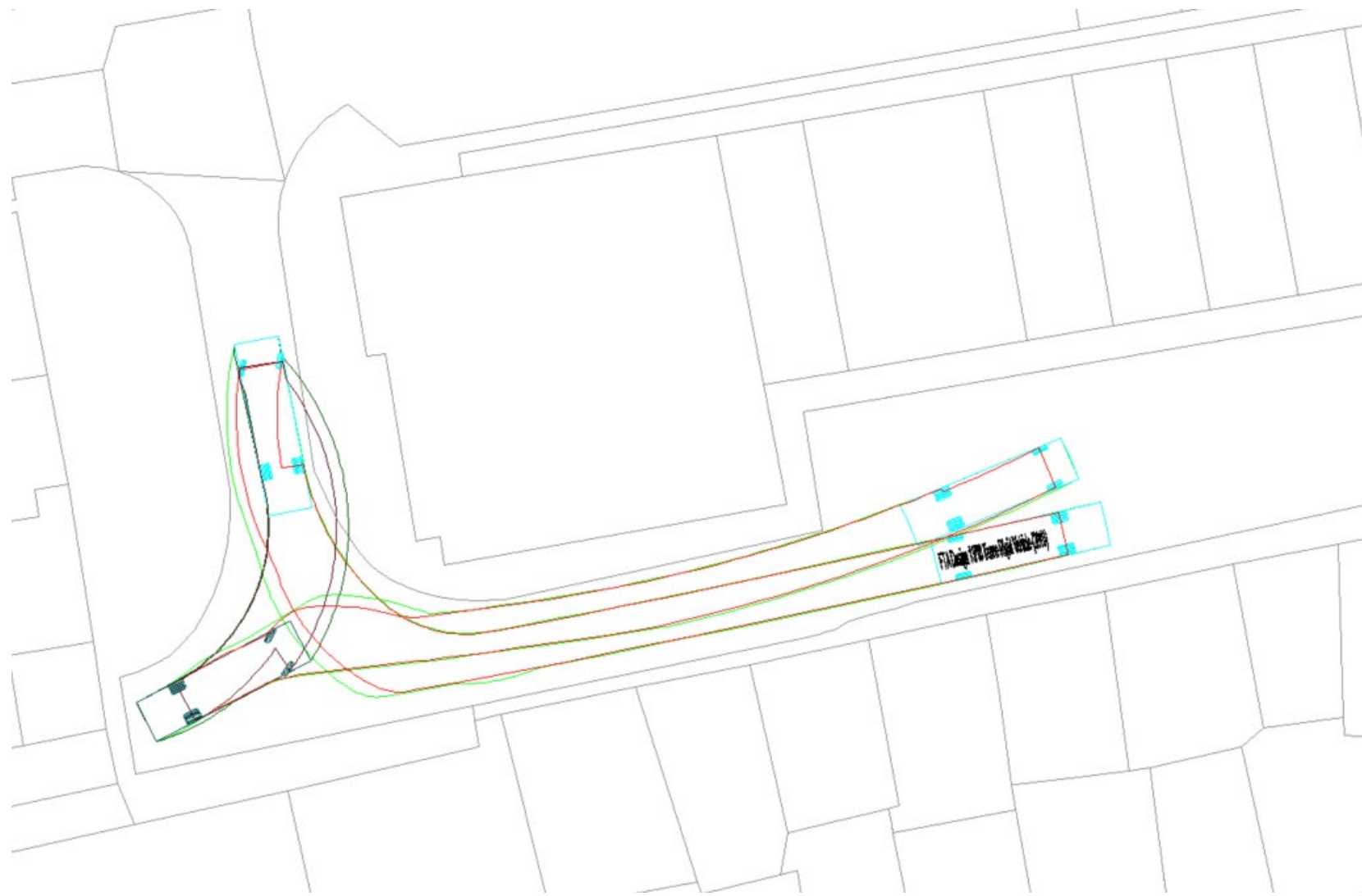
B.23 – 10m Rigid Lorry three point turn
