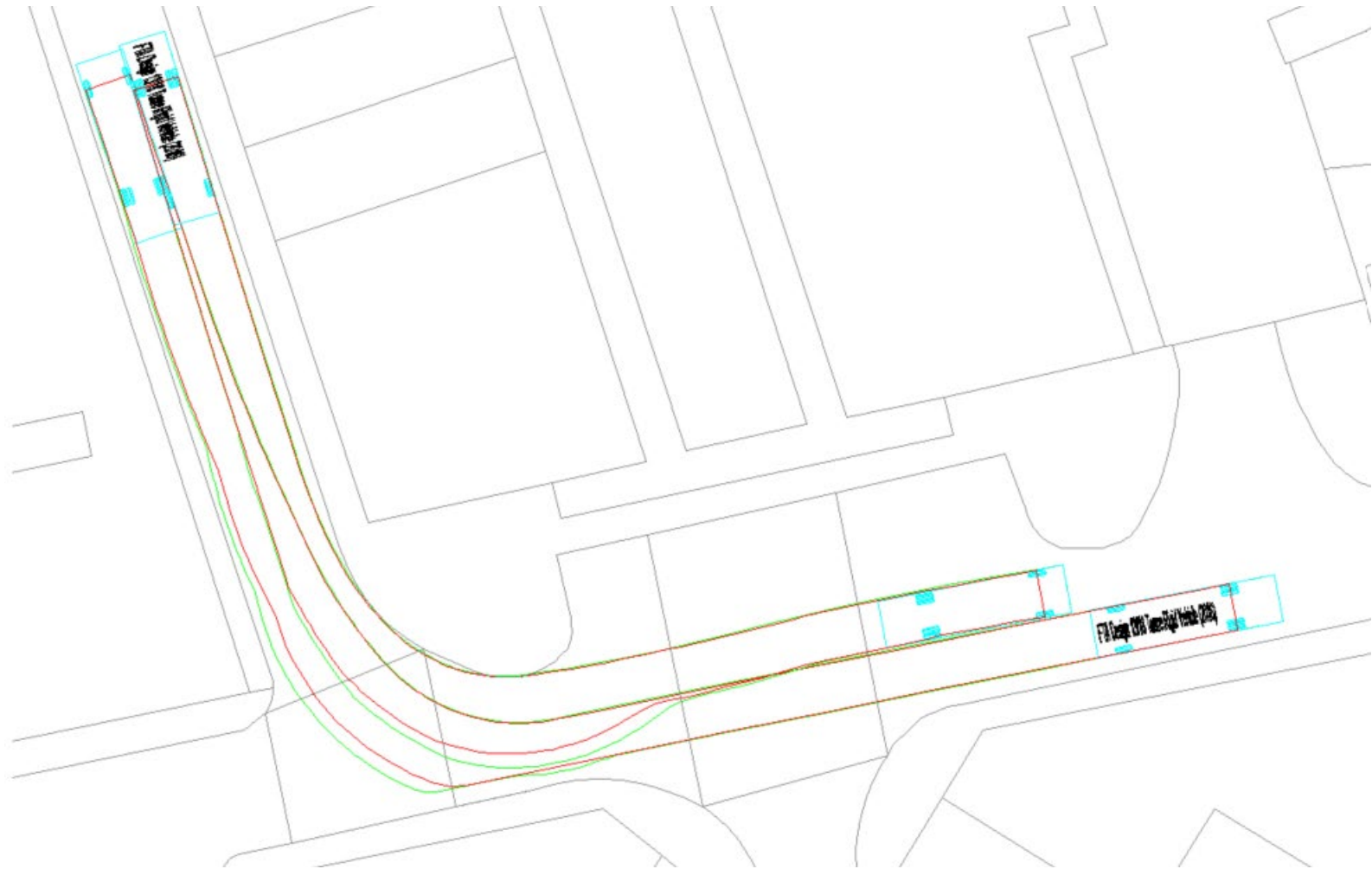
B.16 – 10m Rigid Lorry at Easter Drylaw Place Junction: Left out / Right in
