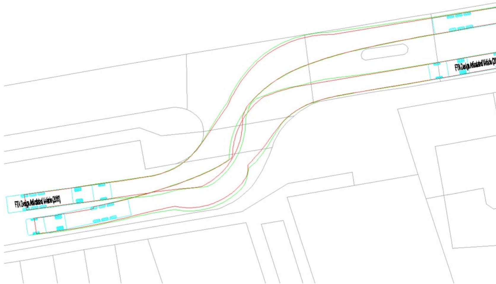
B.2 – Articulated Lorry at Ferry Road Junction: Right out / Left in
