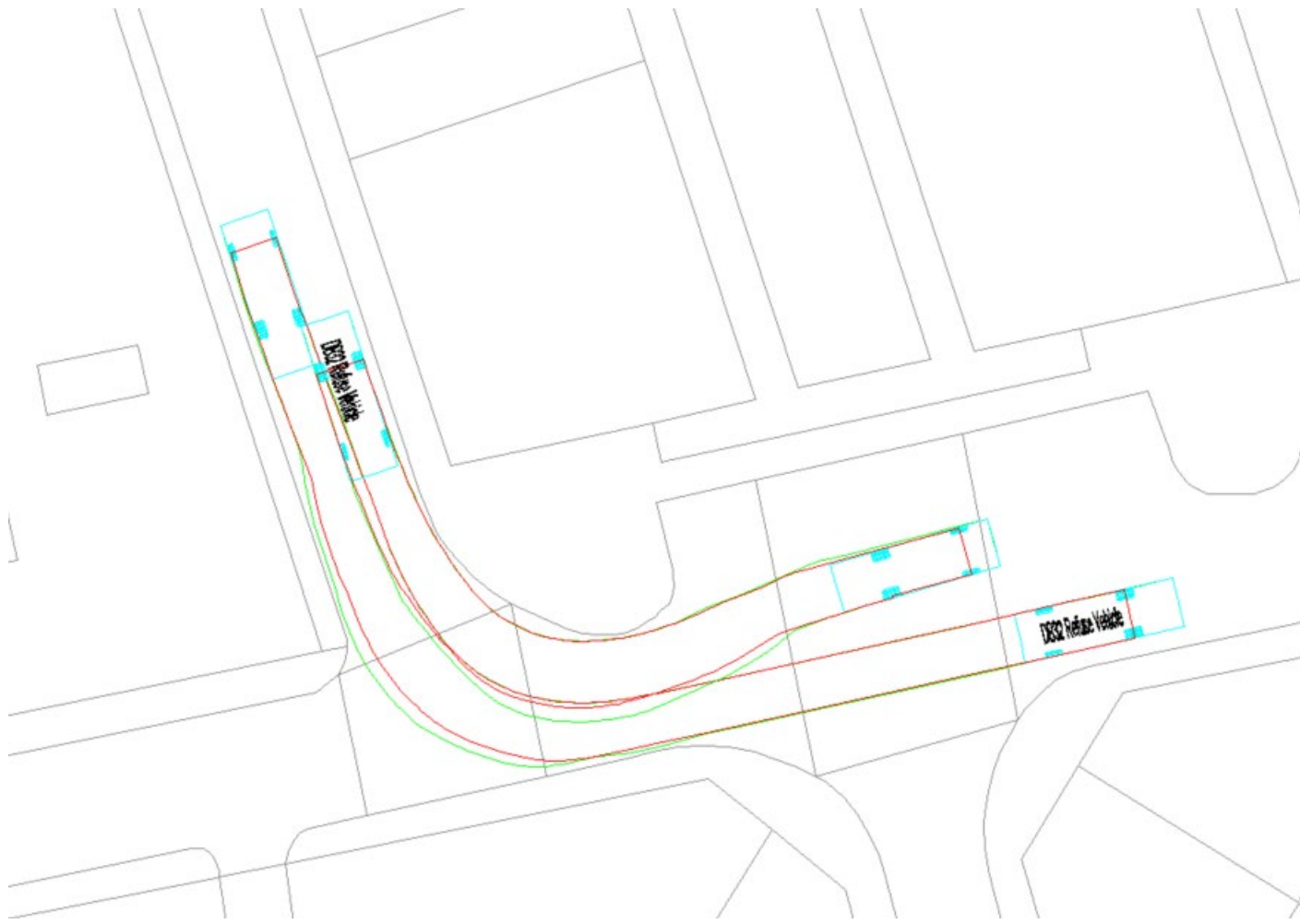
B.12 – Refuse Vehicle at Easter Drylaw Place Junction: Left out / Right in
