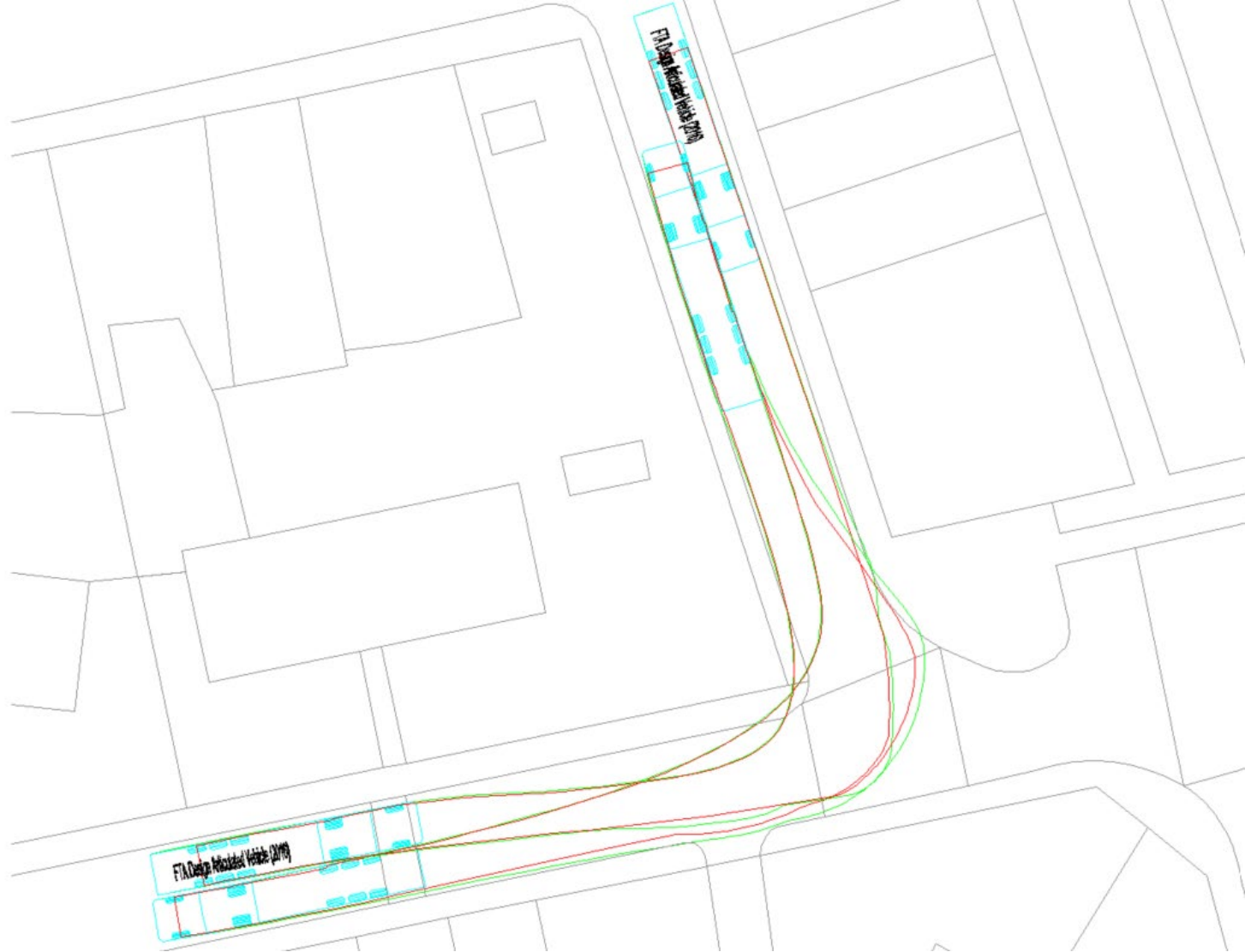
B.9 – Articulated Lorry at Easter Drylaw Place Junction: Right out / Left in
