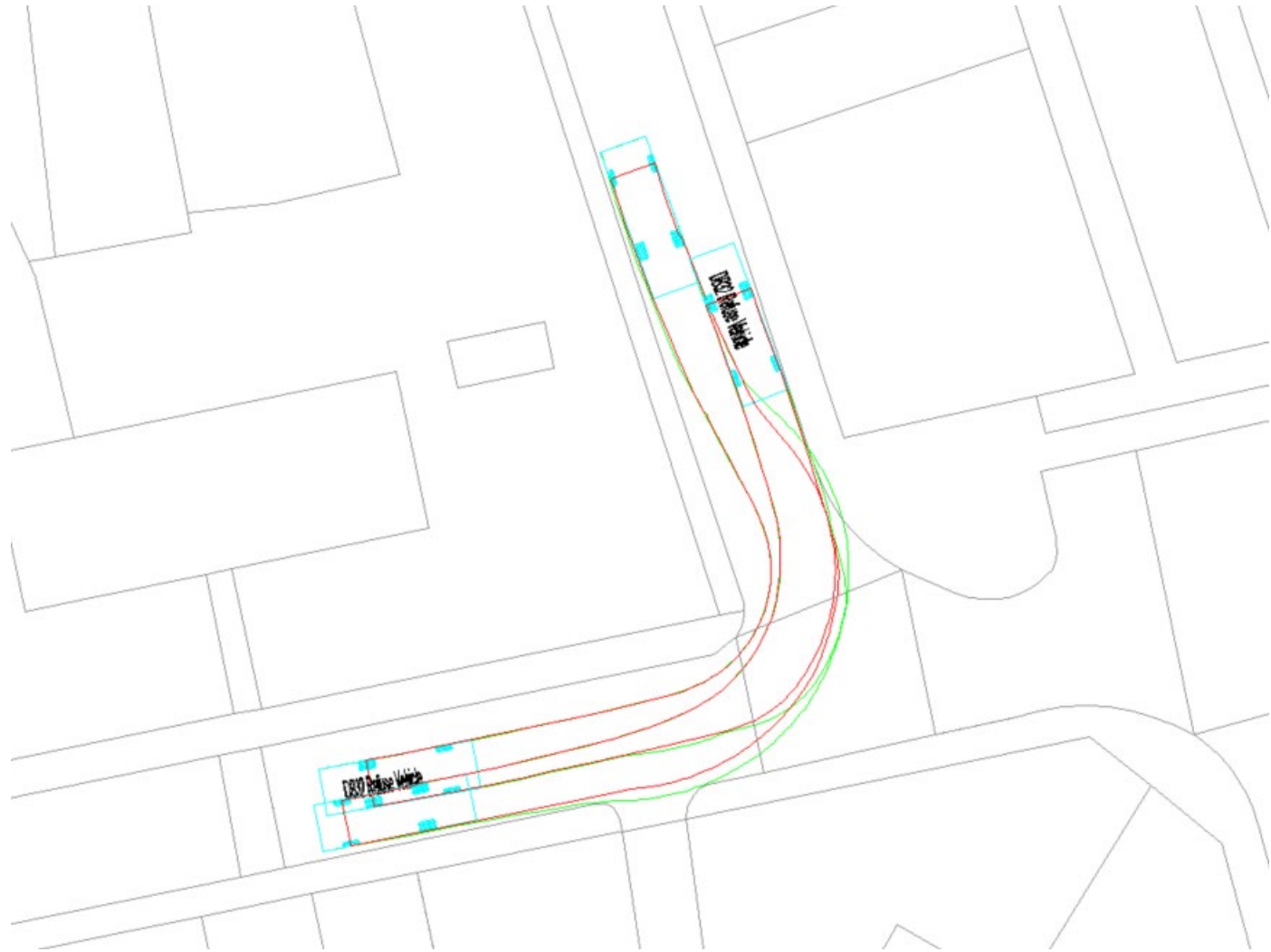
B.11 – Refuse Vehicle at Easter Drylaw Place Junction: Right out / Left in
