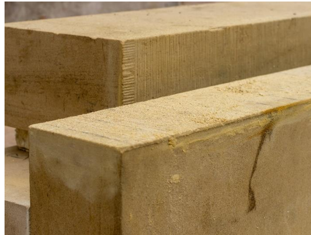
Sandstone blocks for stone repair
