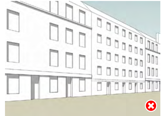
Windows too small? - While the five storey tenement has the same eaves height it has much smaller windows than those of neighbouring tenements. The small scale creates an inharmonious relationship.
