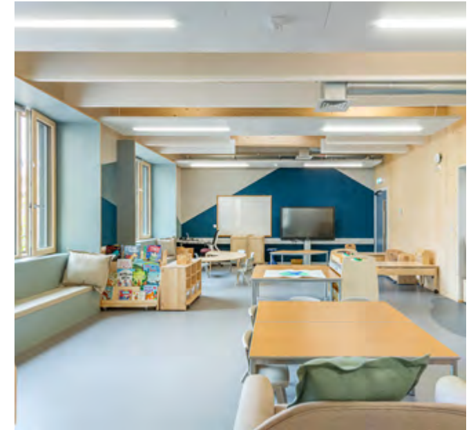
Minimising embodied energy of new buildings - The extension to Sciennes Primary School was constructed using stone-clad exposed cross-laminate timber (CLT). The use of CLT minimised the embodied energy by using natural materials that contribute to carbon storage. By exposing the CLT internally a comfortable environment was created without needing additional internal finishing. The extension was also designed to Passivhaus standard, reducing the operational energy consumption of the scheme. The external stone cladding responded to the setting of the extension next to a category B listed building in the Marchmont Conservation Area. Photos courtesy of Holmes Miller, © Chris Humphreys Photography.
