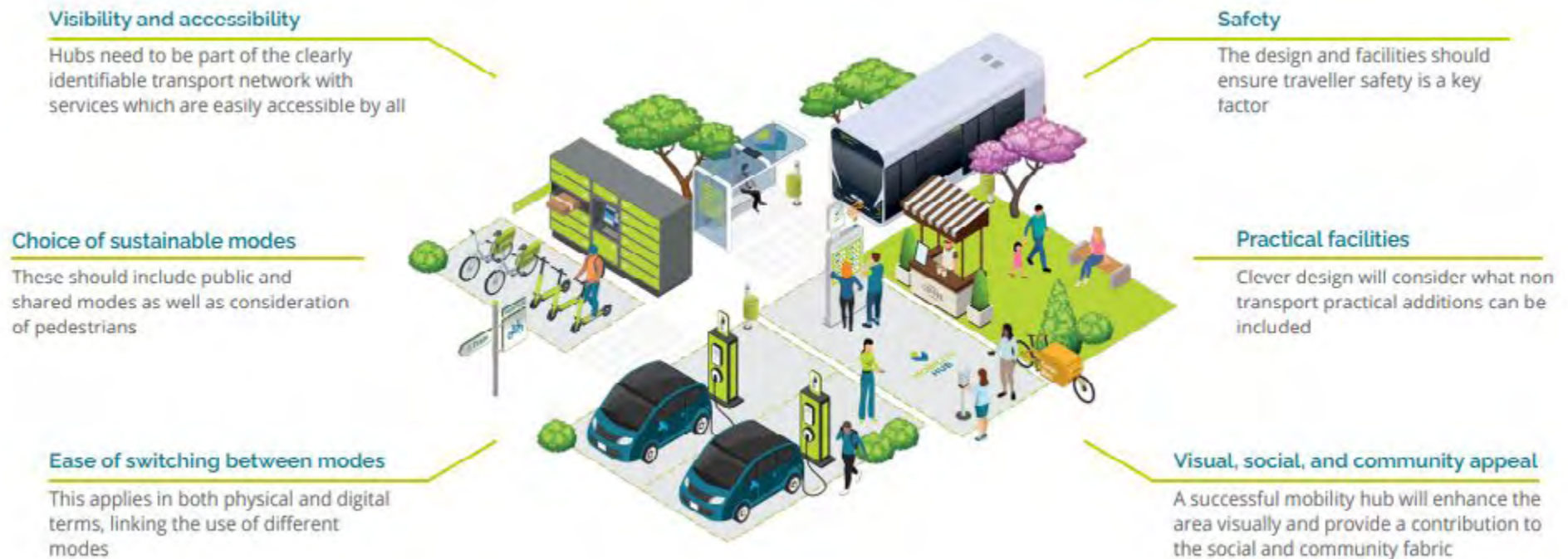
Designing a Mobility Hub - The diagram above shows the six key factors to consider in the design of a mobility hub. Diagram from CoMoUK.
