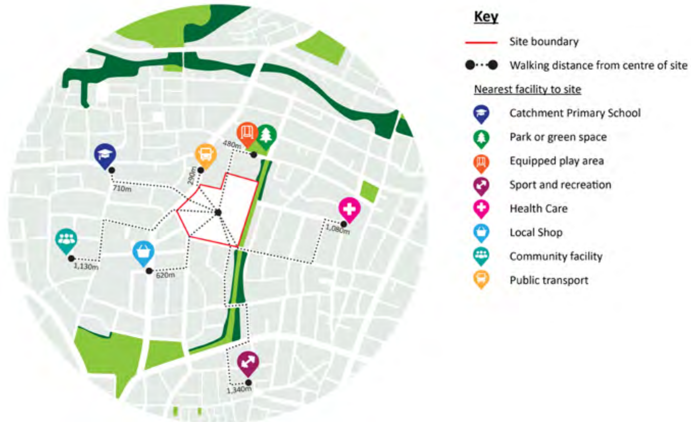
Measuring Walkability Ratio - This example has a walkability ratio of 5/8, as five of the eight key facility categories are within the appropriate distance of the centre of the development.
