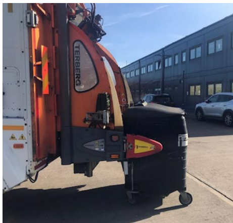
Figure 1 Bin on bin lifting gear at rear of refuse collection vehicle
